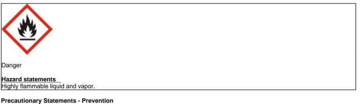
Use explosion-proof electrical/ ventilating/ lighting/ equipment. Keep away from heat, hot surfaces, sparks, open flames and other ignition sources. No smoking. Keep container tightly closed. Ground and bond container and receiving equipment. Use only non-sparking tools. Take action to prevent static discharges.
